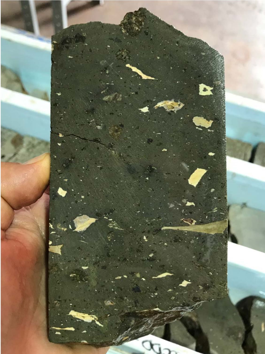
(Figure 3: Diamond drill core sample of the mafic tuff marker bed. This unit has been identified in most drill holes completed at Comet Well to date demonstrating the strong continuity of stratigraphy within the targeted area.)
