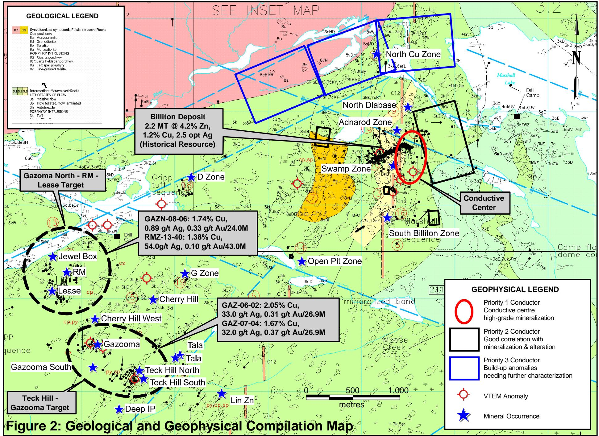
**Figure 2: Geological and Geophysical Compilation Map**
