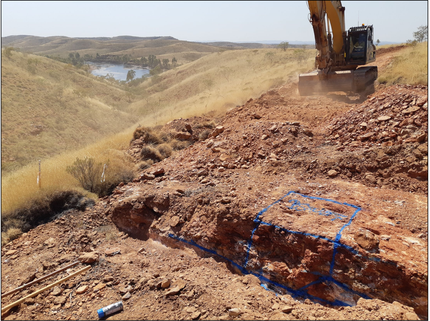
(Figure 3 – Photograph showing the location of a gold-bearing conglomerate horizon from bulk sample BSX057 at Beatons Creek before sampling.)
