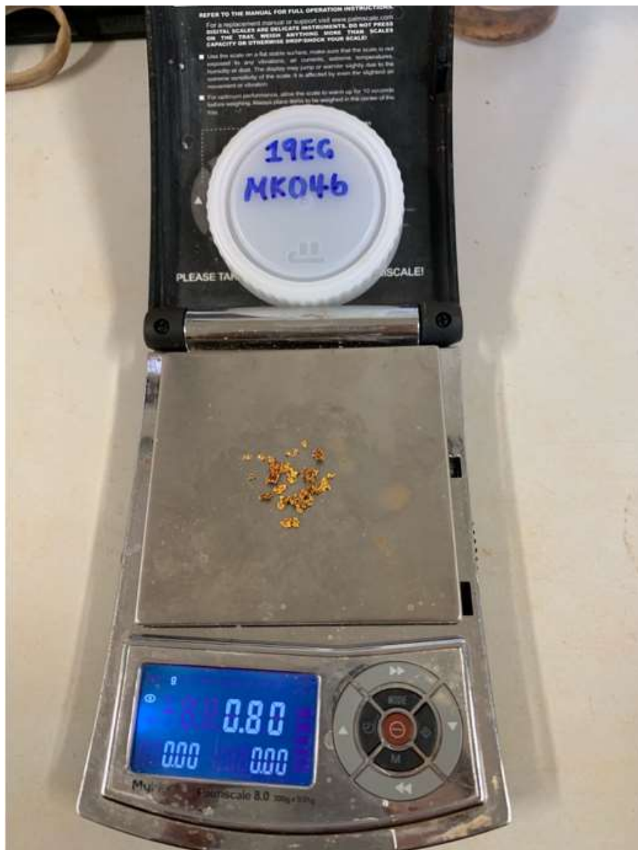
(Figure 8: Gold grains recovered from a test pit at Paradise. Local gold sources may include veins in basement in this location. Like gold found on the Egina mining lease 14 km south-southwest of Paradise, a mechanical sorter could readily recover all such gold grains. These concentrated samples of selected material are not necessarily representative of mineralization hosted on the Egina property.)
