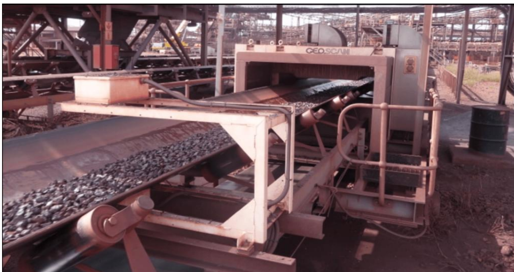
Exhibit 8: Conveyor-Based Sensor Ore Sorting System. Source: Company Website
