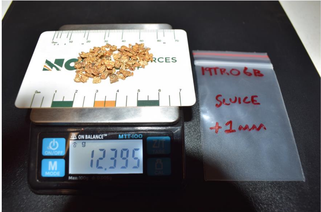
(Figure 2: 12.395 grams of gold from 6B sluice +1mm (subset of 40.9 grams total).)
