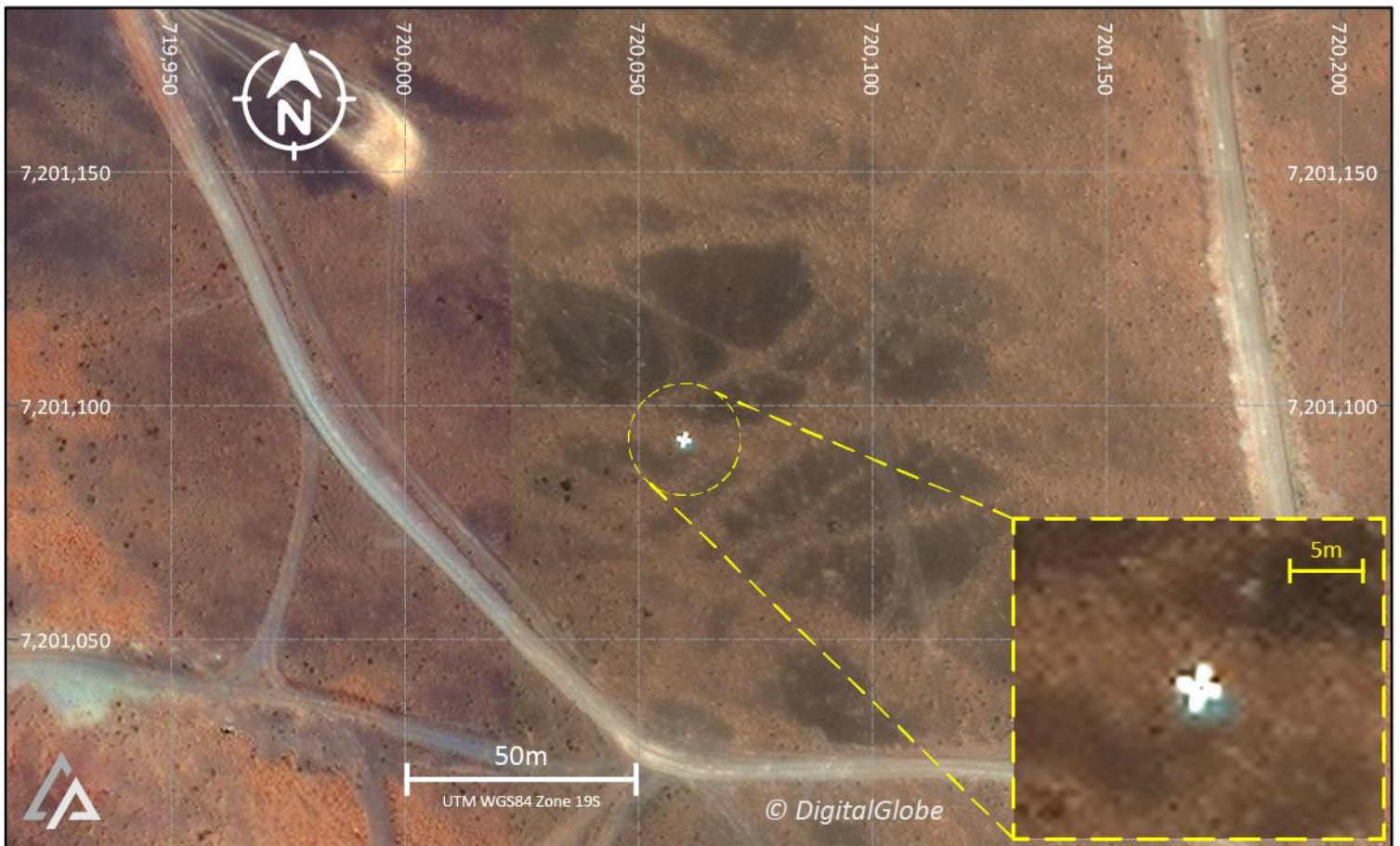
Figure 1 - Plan view showing one of the ground control points (GCPs) used for the PhotoSat surveying.
