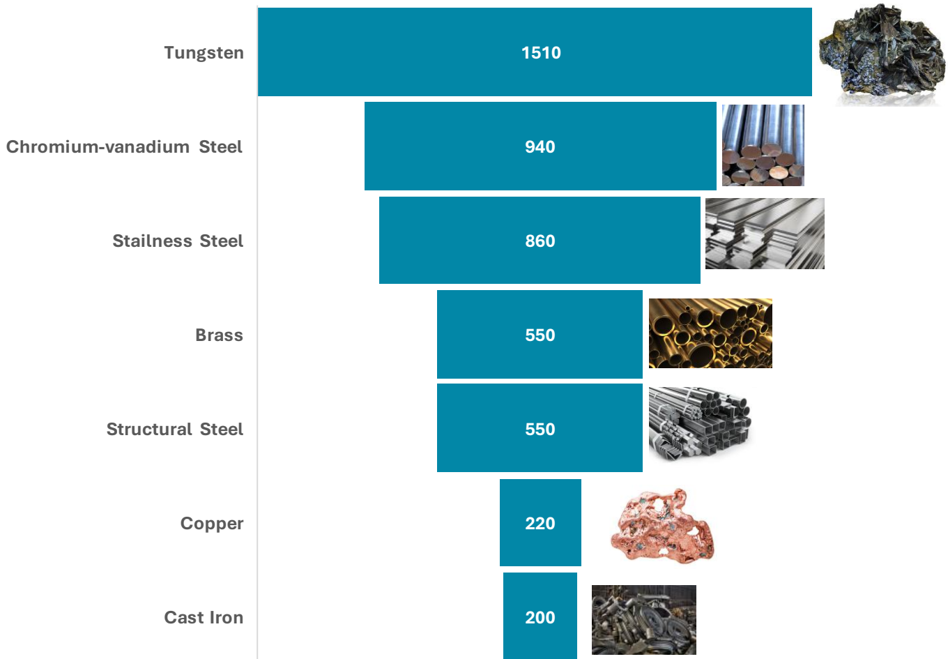
Exhibit 18: Tungsten Tensile Strength vs Other Metals (in megapascals). Source: Diamond Equity Research
