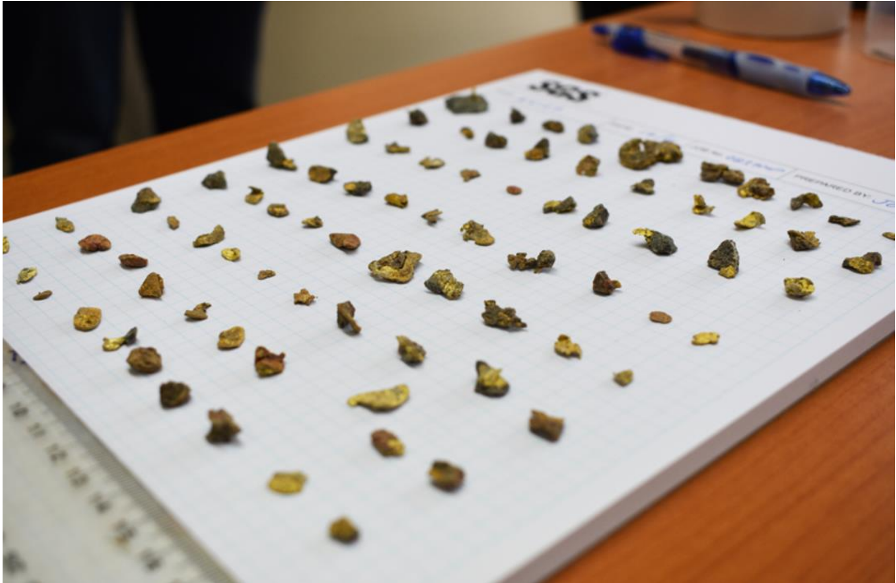
(Figure 3: Gold nuggets recovered from bulk sample KX157. Blue gridlines are 5 mm. Most nuggets are rounded and flattened, a clear indication of a water-worn alluvial origin.)
