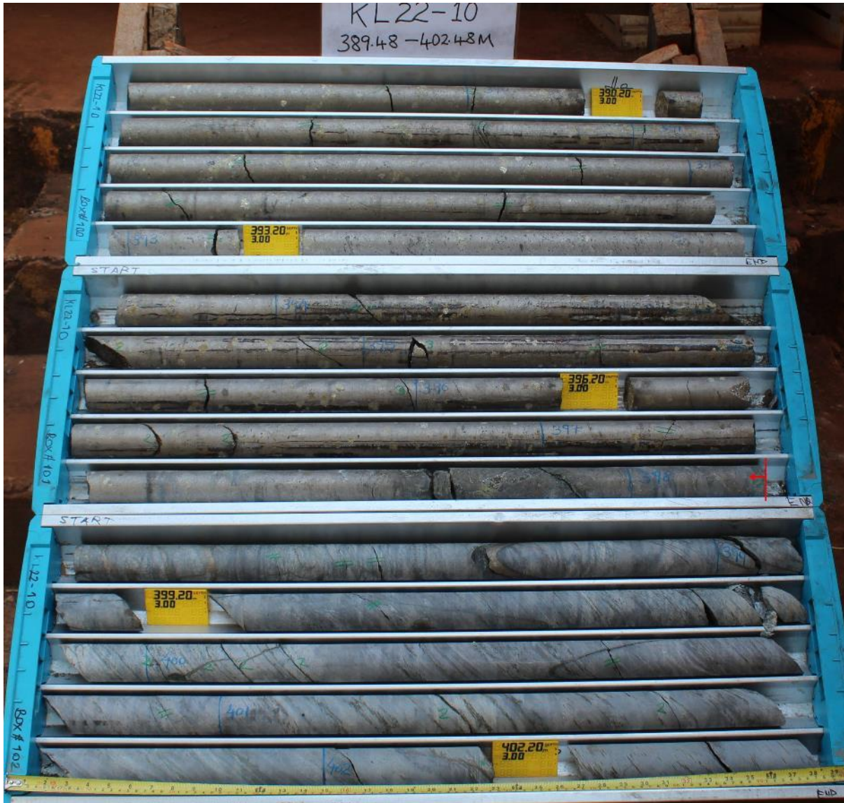
Figure 5 Core Photo showing Massive Sulfide Mineralisation in KL22-10 Mineralised Interval 389.48–398.18 m = 8.7 m at 2.77% Ni, 0.46% Cu, and 0.24% Co, (3.63% NiEq23) (end of mineralised interval shown by red arrow)
