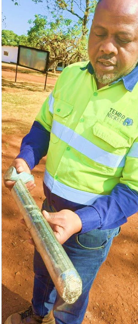
Figure 8 Jumbe Maulid (Geology Superintendent) from TNCL showing Massive Sulphide in Drill Core from Hole KN22-03 at North Zone, which intersected 52.0 m at 2.37% Ni, 0.25% Cu, and 0.14% Co, (2.85% NiEq23)
