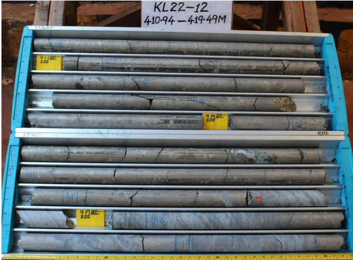
Figure 7 Core Photo showing Massive Sulfide Mineralisation in KL22-12 Mineralised Interval 410.94–417.57 m = 6.63 m at 2.81% Ni, 0.45% Cu, and 0.19% Co, (3.51% NiEq23) (end of mineralised interval shown by red arrow)
