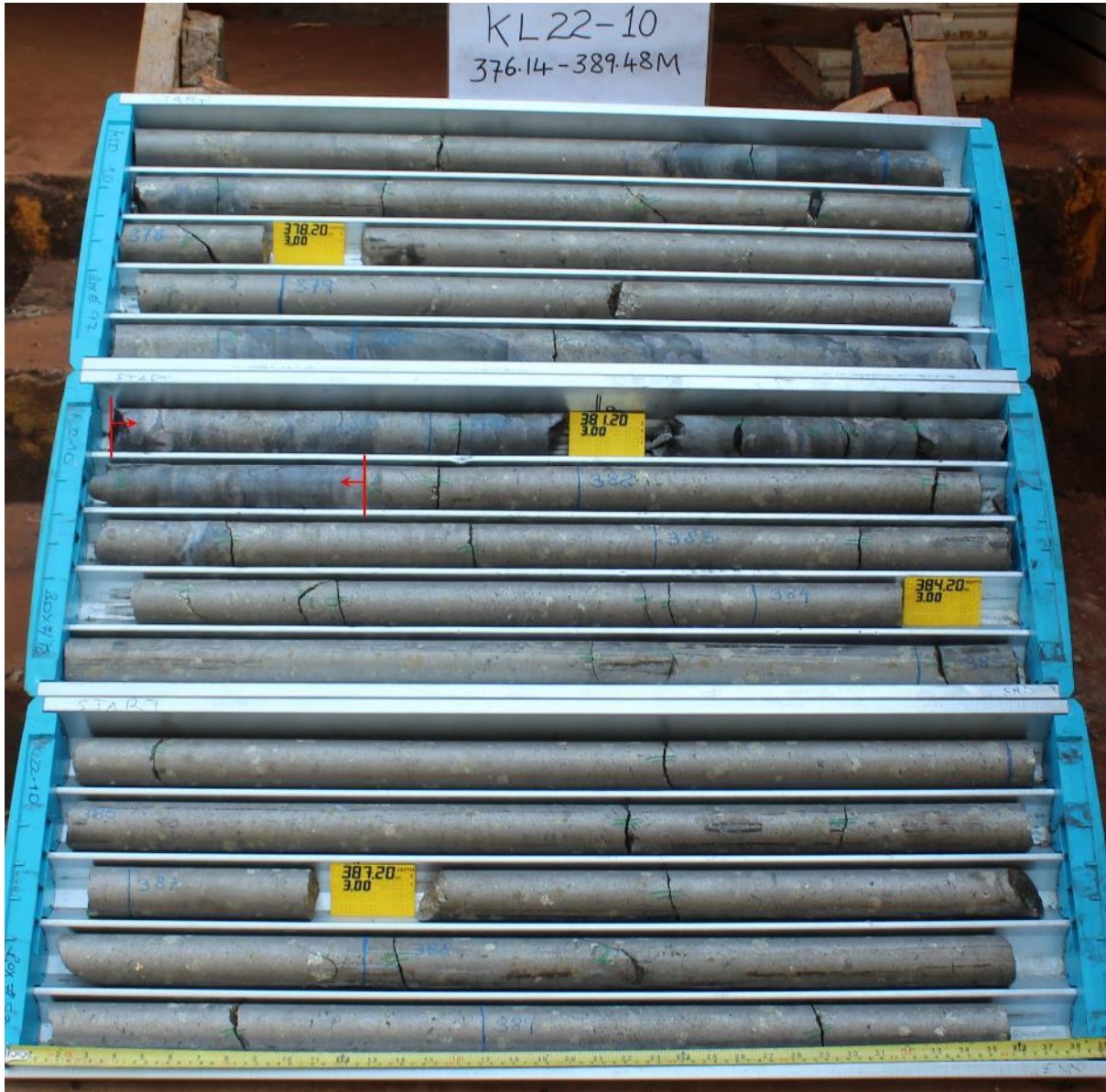
Figure 4 Core Photo showing Massive Sulfide Mineralisation in KL22-10 Mineralised Interval 376.14–389.48 m = 13.34 m at 2.56% Ni, 0.44% Cu, and 0.20% Co, (3.28% NiEq23) (includes 0.96 m of internal waste (<0.58% NiEq23) 380.82–381.78 m (shown by red arrows))
