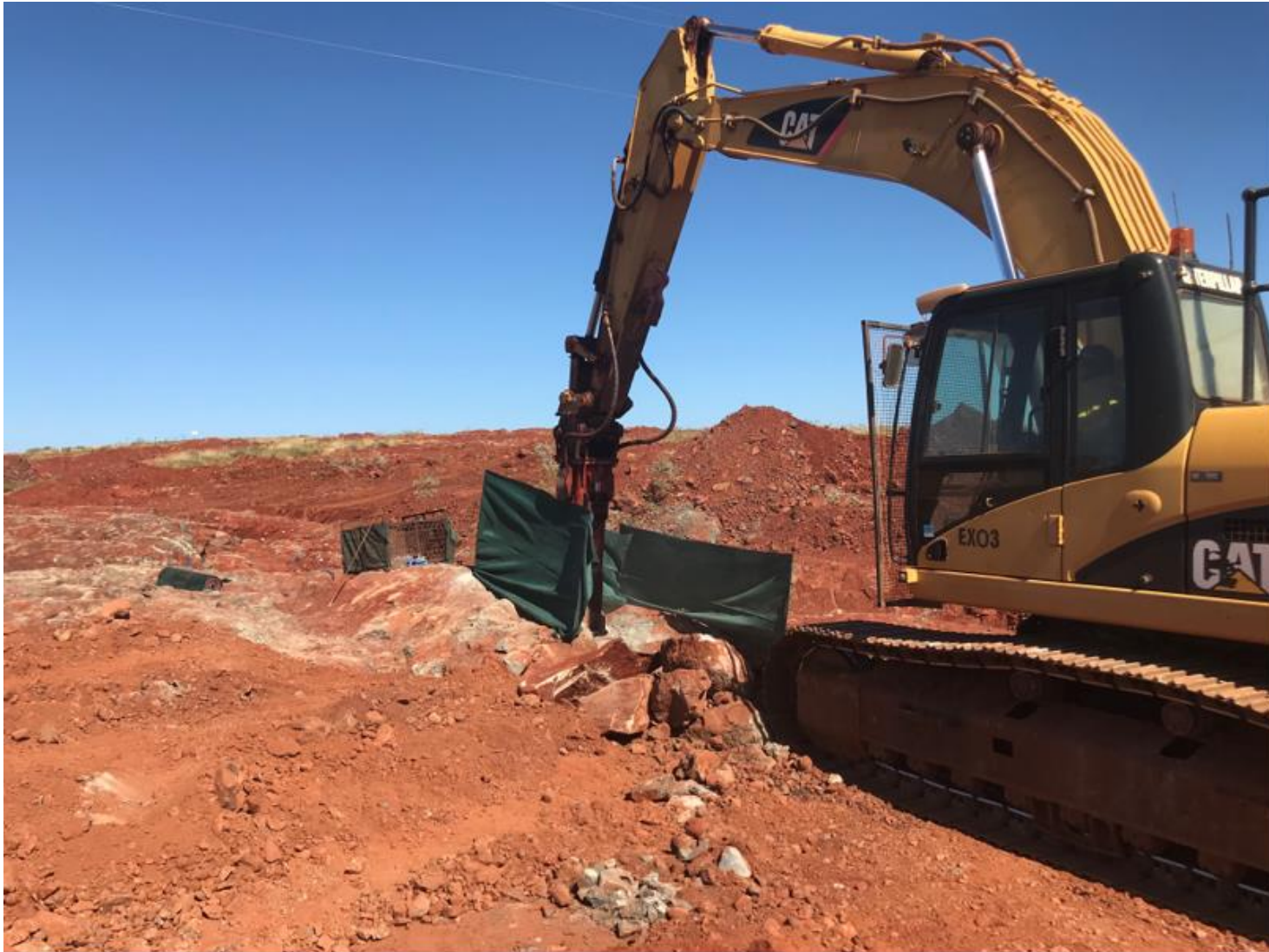
(Figure 2: Sample extraction at Comet Well. Screening is used to contain fly rock during sampling. A chiselmoil on a rock breaker is used to produce sample material.)
