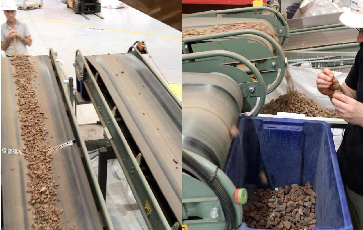
(Figure 2 – Left, looking down on the conveyor discharge from the TOMRA ore sorter. The conveyor on the left is reject material and that on the right carries a very small fraction of concentrate. Right, discharge bins, concentrate in the foreground and reject in the background.)
