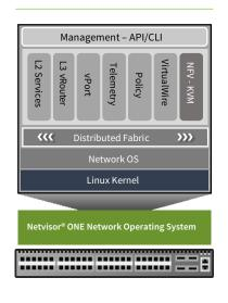
Netvisor OS provides a modular, resilient software design with advanced Layer 2 and 3 networking and services
