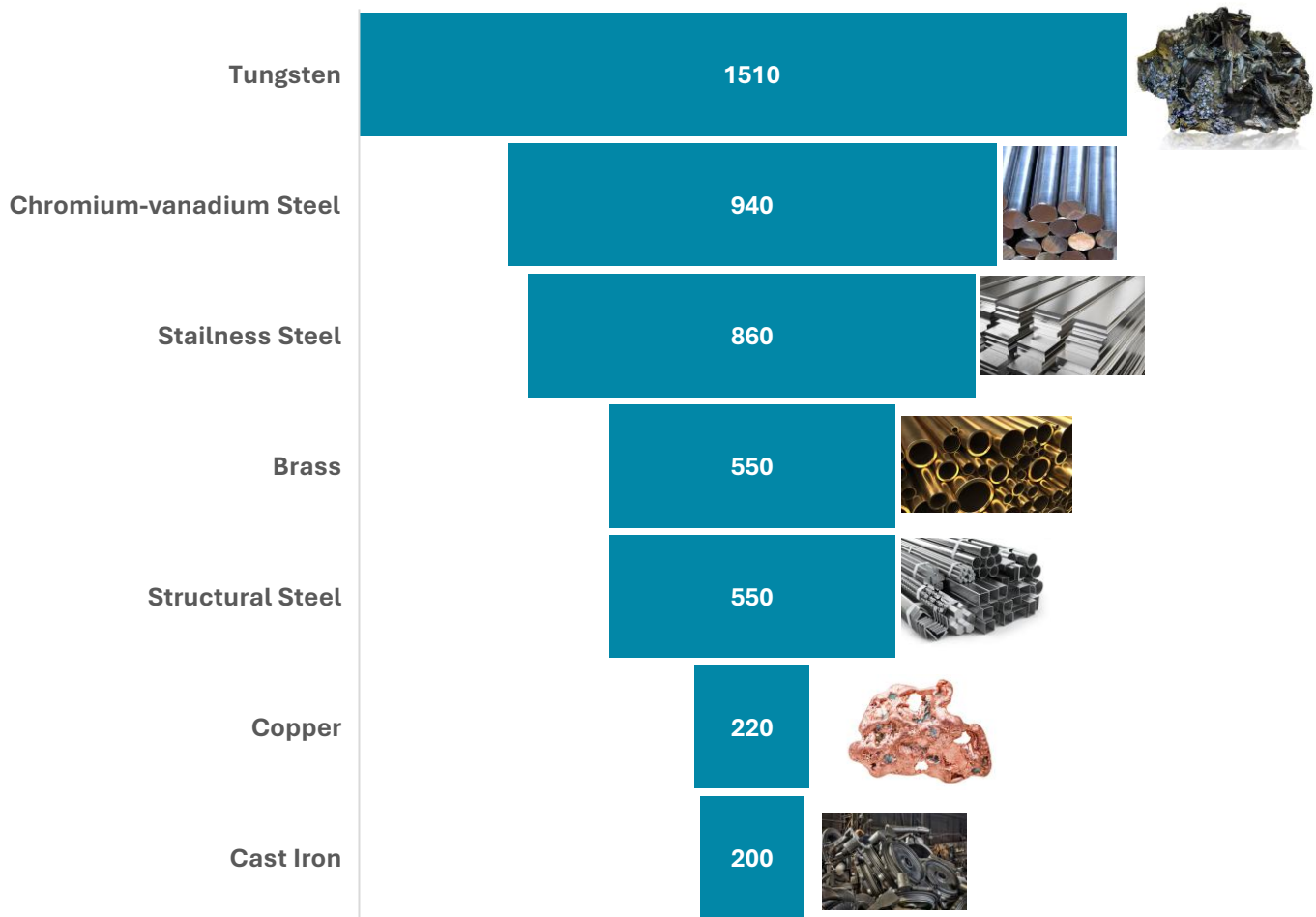
Exhibit 24: Tungsten Tensile Strength vs Other Metals (in megapascals). Source: Diamond Equity Research
