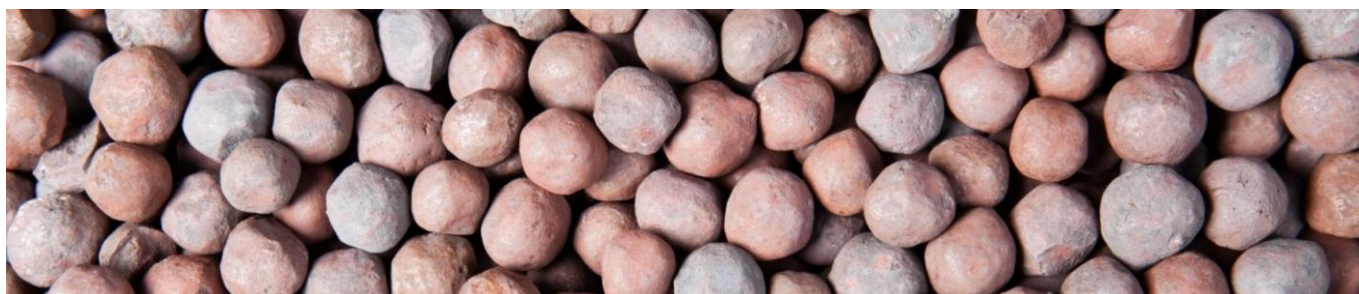
Exhibit 27: High-Grade DR Pellets for DRI and EAF Steelmaking Applications. Source: Mesabi Metallics
