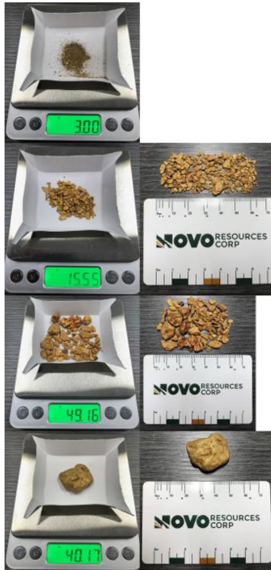
(Figure 2 – Gold produced from the first bulk sample at Egina. Top: Fine gold panned from tabled Falcon concentrates. Second row: Small nuggets captured by the Falcon concentrators. Third row: Coarse nuggets captured in discharge sluice. Bottom row: Large gold nugget found when detecting oversized material. In total, 107.88 grams of raw gold were produced from 95 bench cubic metres of gravel. X-ray fluorescence analysis of gold nuggets indicate gold purities ranging from 91-93% with silver making up most of the balance. Container was zeroed on the scale prior to weighing the gold. Please note that gold mineralization in the above photos is not necessarily representative of the mineralization hosted on the Egina property.)
