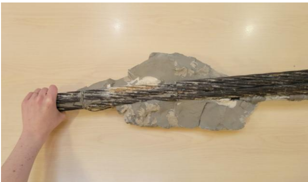
Figure 3: An exhumed tieback sample with steel cables and surrounding grout, 6" in diameter.
