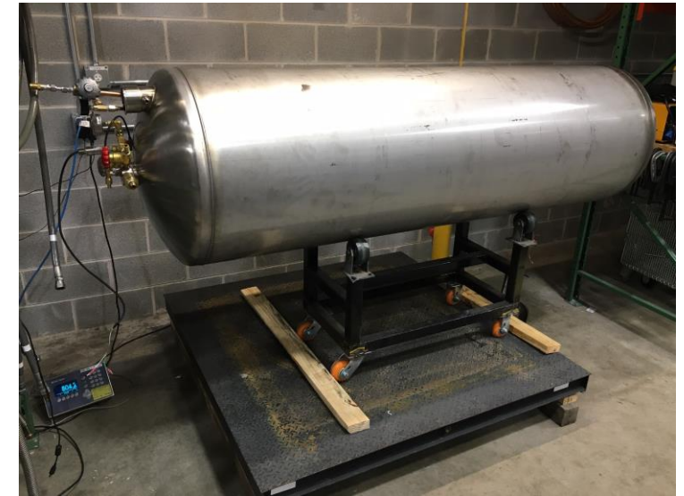
Liquid Hydrogen Onboard Vehicle Tank being tested at our Canton, Georgia (USA) facility
