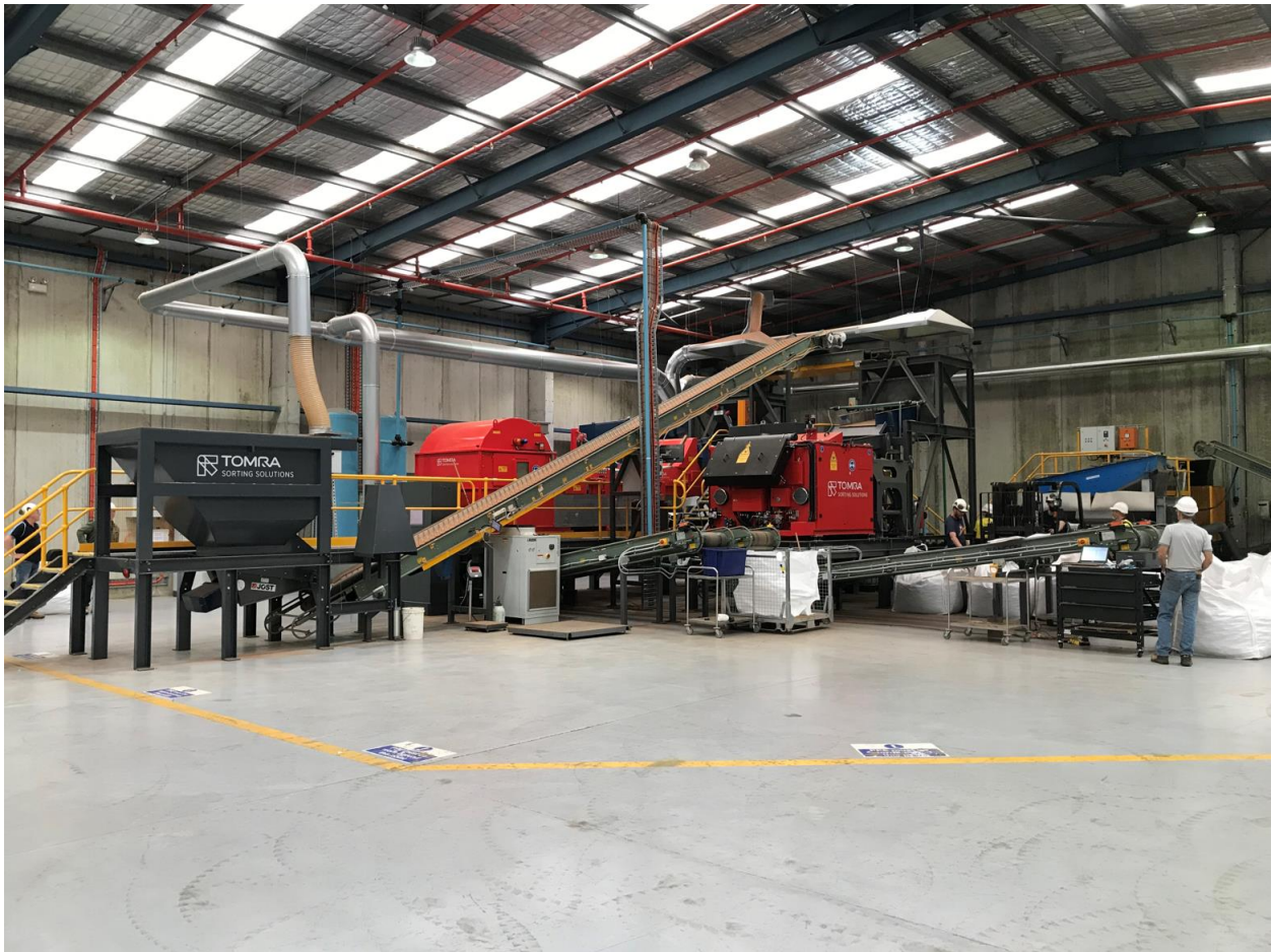
(Figure 1 – TOMRA mechanical ore sorter at TOMRA Sorting Pty. Ltd.'s Castle Hill, New South Wales testing laboratory. This sorter employs XRT to identify rocks containing particles of high atomic mass such as gold and electromagnetic induction EM to identify rocks with a propensity to become electrically charged due, occasionally, to the presence of metallic particles.)
