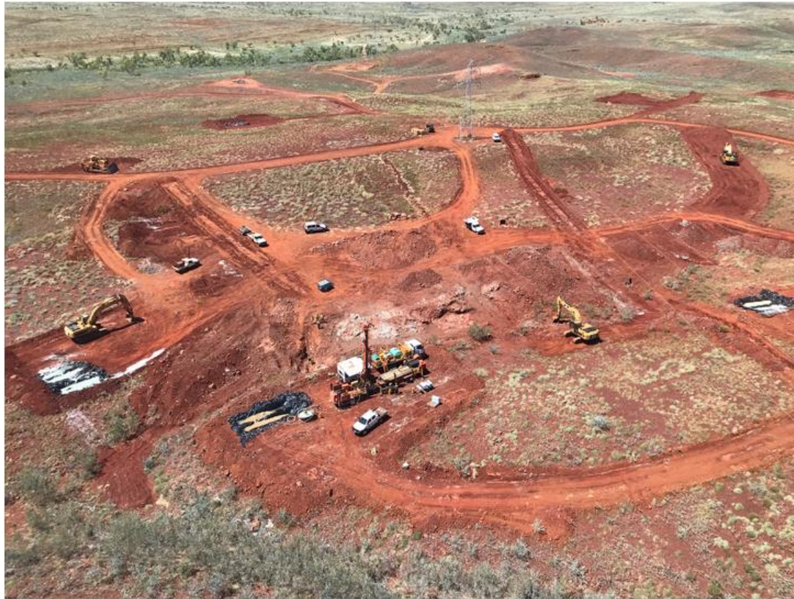
(Figure 2: Aerial photograph of the Powerline showing looking southwest. The first trench to expose bedrock is immediately behind the mast of the diamond core drill. Numerous detector strikes were encountered in multiple layers. The footwall contact of the conglomerate sequence is not exposed in this trench. In situ gold nuggets as see in Figure 3 have been extricated from rock matrix material.)
