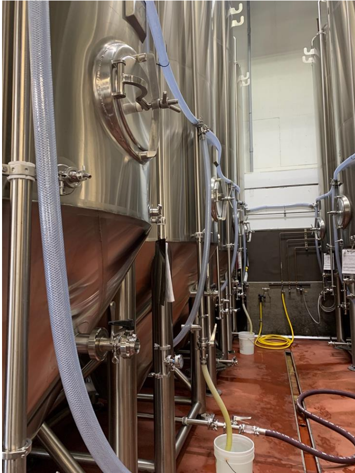
PVC tubing half-way up tanks to enable easy clean and visual inspection
