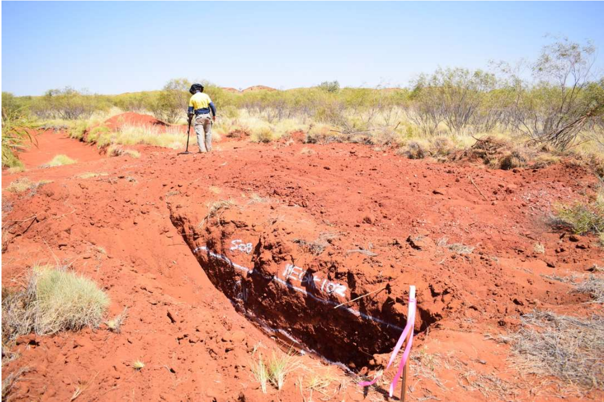
(Figure 2: Typical test trench. To explore new areas, Novo digs pits such as these at 50 m spacing. Geology of the gravel profile is recorded, the pit bottom and spoils piles surrounding the pit are metal detected for nuggets, and a small 0.5-1 tonne mini-bulk sample is collected for processing. Such bulk samples are indicative only and only used to evaluate presence of gold. Multiple pits at both the South Egina and Paradise targets have yielded appreciable gold through detecting and/or mini-bulk sample processing. See Figure 5-7.)
