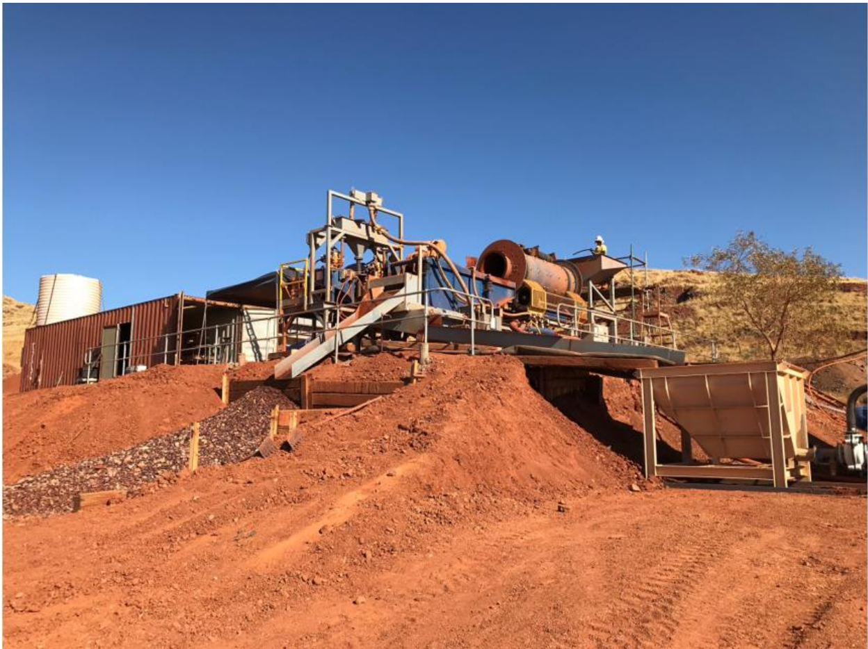
(Figure 1 – Novo’s IGR3000 gravity gold plant in operation at Egina. Plant capacity is about 25-35 tonnes per hour. Falcon centrifugal concentrators, top middle, are employed to capture gold. A discharge sluice exits the plant on the right. Oversize material forms a pile on the left. This plant is ideally suited for treating large bulk samples of terrace gravel as part of Novo’s program of exploring this expansive target. Protocols for sampling and processing have now been fully established in preparation for a much larger program treating similar-sized bulk samples in 2019 with the intent of establishing a first ever resource for the project. Plans are also being made for large-scale test sampling.)
