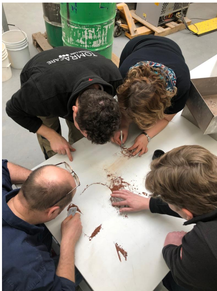
(Figure 2: TOMRA personnel hand sorting 7.17g of nuggets from 35.5g of concentrate, retrieving all 120 nuggets.)
