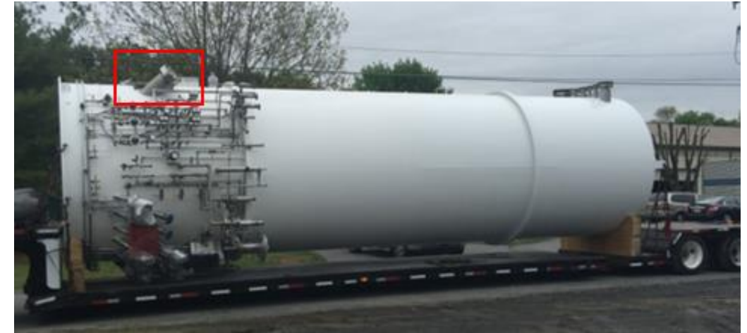
10 ton/day Liq. H2 Cold Box Loaded for Shipment
