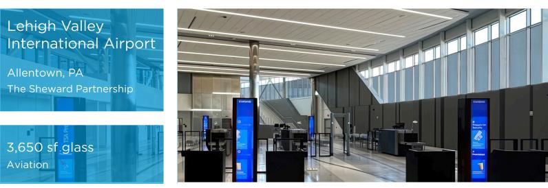
HALIO's electrochromic window technology will automatically darken the windows on hot, sunny days, and let in more light on cold winter days. The technology will help the airport use less energy for air conditioning and heating and should provide about 27% in energy savings per year.
