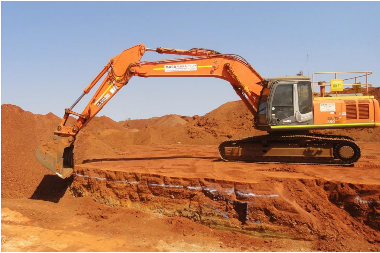
(Figure 1 – Excavation of a 170 tonne bulk sample of gold-bearing lag gravels at Egina. Sand and soil is first stripped off the targeted gravel layer. Yellow material at the base of the bench is weathered sedimentary rock belonging to the Mallina Formation comprising basement in this region. The targeted gravel horizon rests on top of the Mallina Formation and beneath the white line.)
