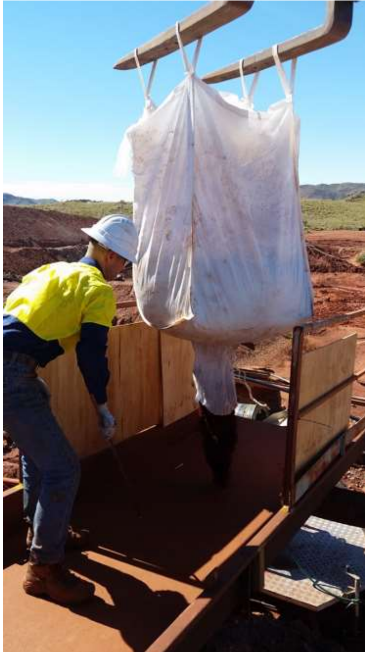
(Figure 4: A mini-bulk sample from a test trench being loaded into a hopper that feeds material into the MAK plant.)
