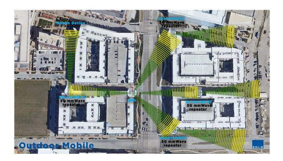
In-building 5G mmWave mobile coverage is not practical with an outside-in macro-cellular approach because high band signals do not penetrate buildings. RocketWAVE™ receives 5G mmWave signals from a rooftop or wall mounted donor antenna and repeats the signals to antennas inside the building.
