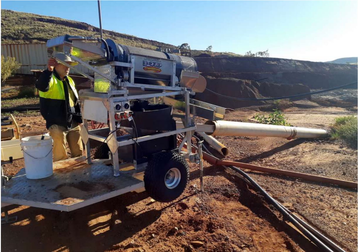
(Figure 3: Mobile alluvial Knudsen (“MAK”) unit capable of processing a mini-bulk sample in approximately one hour. The concentrating bowl is the black circular object near the center. Concentrates are carefully panned after processing each sample, and gold grains and sizes are recorded.)
