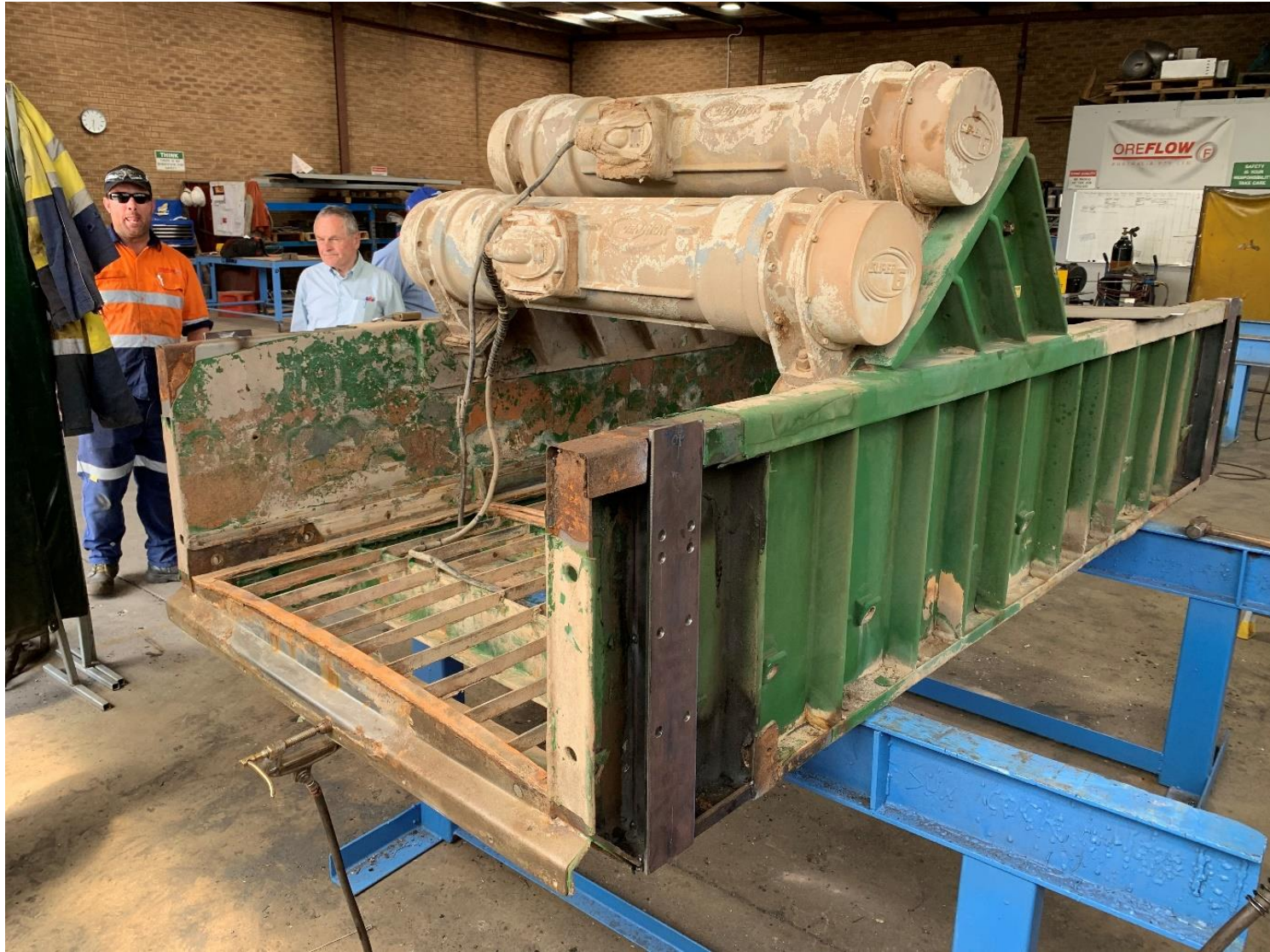
(Figure 2: Trash screen undergoing refurbishment works.)
