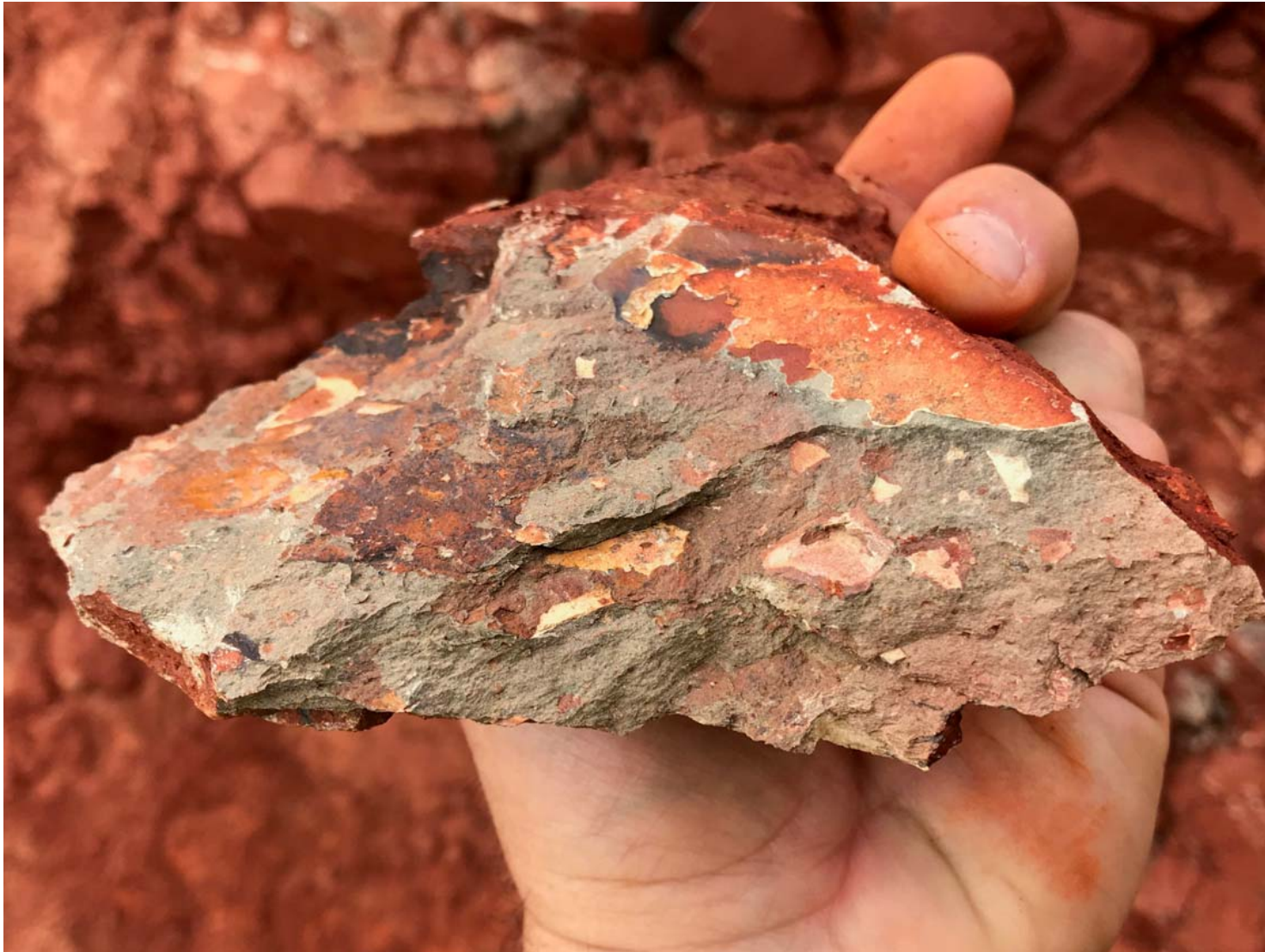
(Figure 2: Sample of mafic tuff, a marker unit closely associated with the upper gold-bearing conglomerate at Comet Well. The ash matrix of the rock appears mafic in composition whereas the light-colored lapilli are of more felsic composition.)
