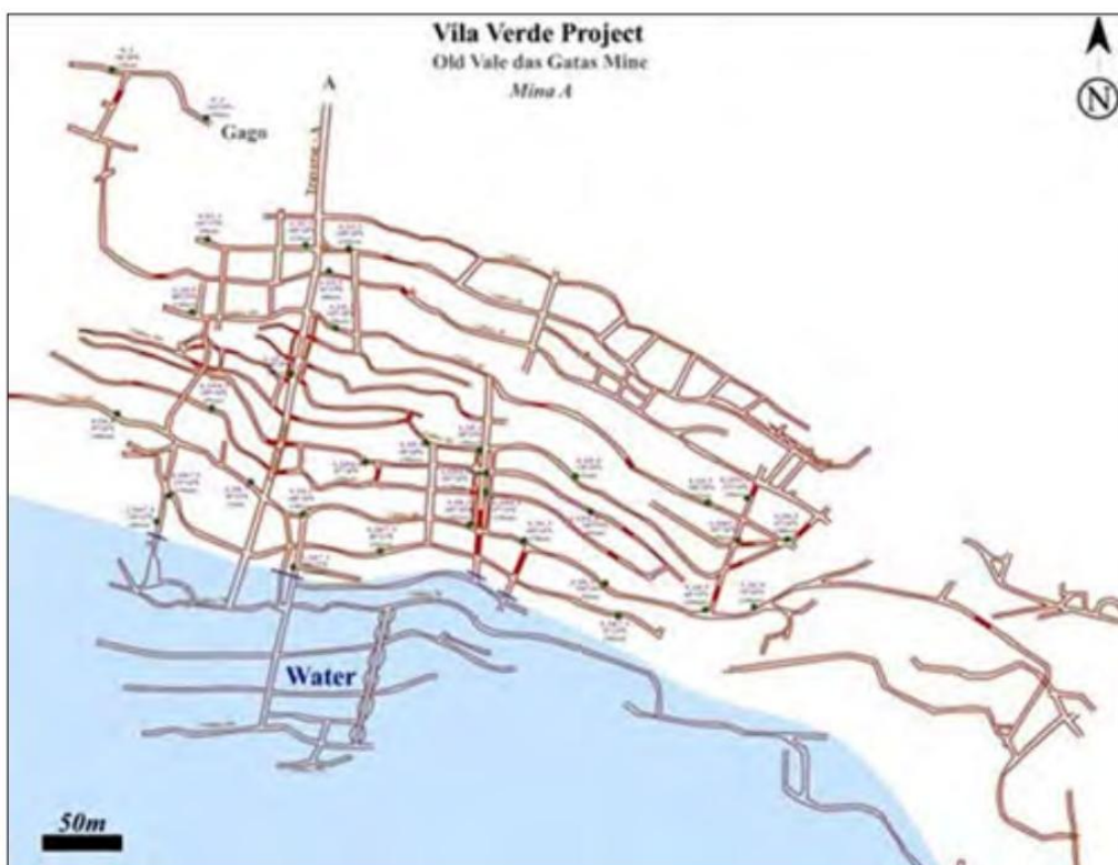
Exhibit 14: Underground Workings of the Vale das Gatas Mine. Source: Technical Report Vila Verde
