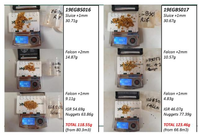
(Figure 2: Various gold nuggets recovered from bulk samples. Virtually all nuggets are rounded and flattened. The photograph is of concentrated gold nuggets and is not necessarily indicative or representative of mineralization hosted on the Egina gold project.)
