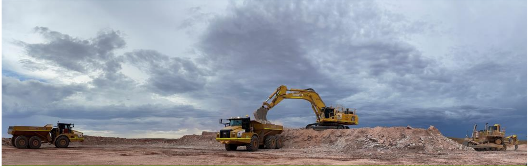
(Figure 3: Cat 745 fleet pre-stripping waste off the Edwards area of Beatons Creek.)
