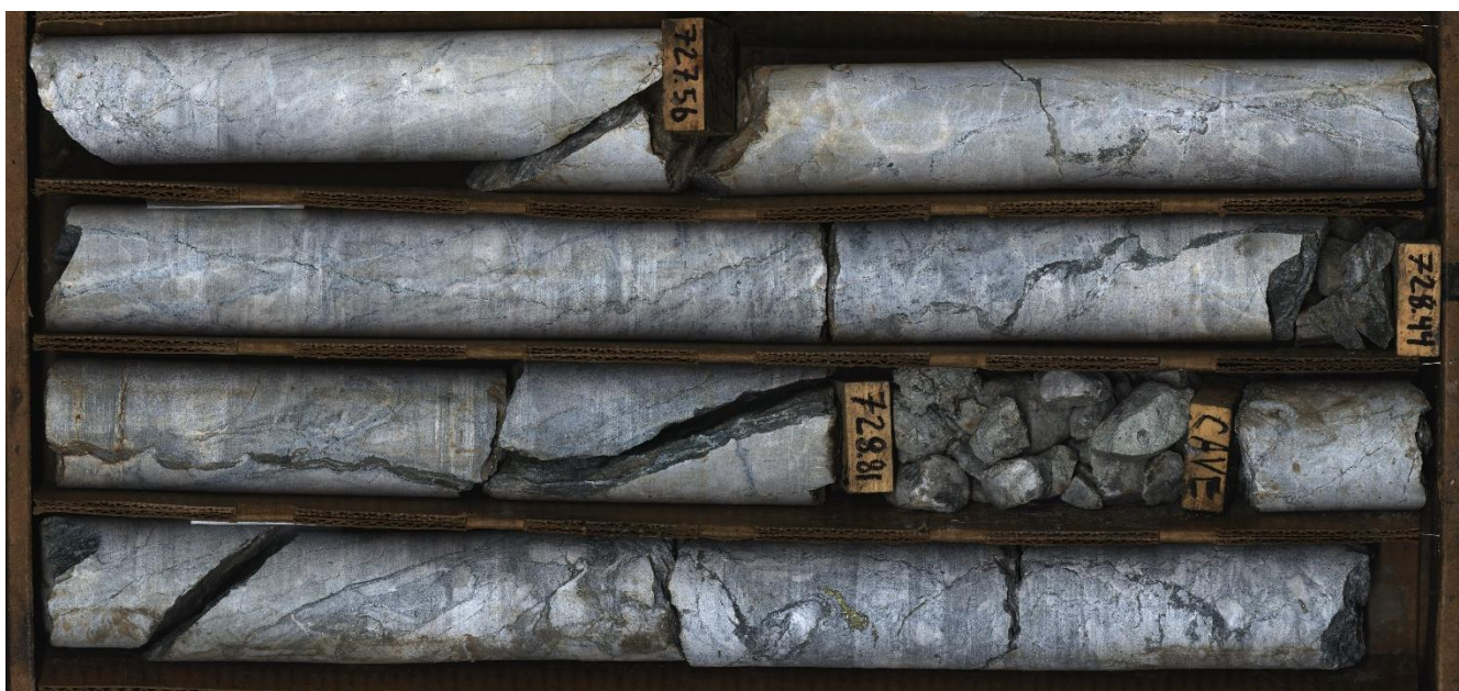
Photo 8. NB26-003; 729 m. Sinuous pygmatic sulfide veinlets and sulfide clots of pyrite-chalcopyrite-molybdenite in high temperature, hydrothermally dolomitized and locally brecciated marble with wollastonite carrying 0.73% CuEq* on 0.18% Cu , 0.15% MoS 2 and 7 g/t Ag .
